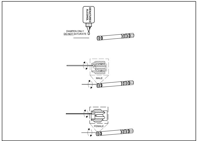
Figure 5. Cleaning Male and Female Connectors
