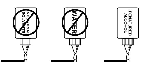
Do NOT use Industrial Solvents or Water on connector. Use only Denatured Alcohol.
