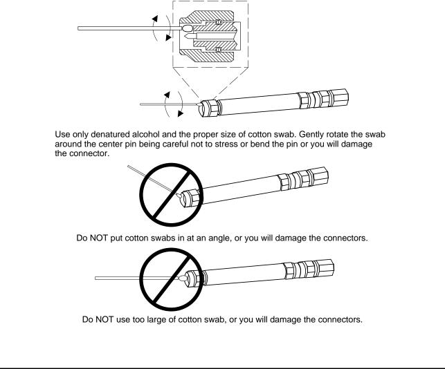
Figure 6. Proper and Improper Cleaning Techniques
